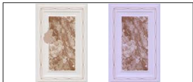
Fig (c) Spot defect
